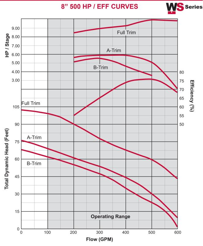
These curves are based on factory tests when pumping clear, fresh, non-aerated water at a temperature not exceeding 85°F. Due to production tolerances, these curves can vary plus or minus five percent.
