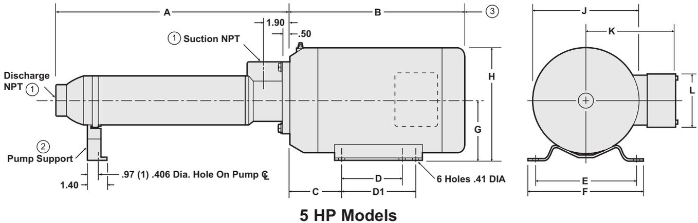
1. The inlet and discharge thread size for C.I. and stainless steel models in the 5, 10, 15 GPM pump sizes is 1" NPT; The 20 and 35 GPM pump size is 1 1/2" NPT.
