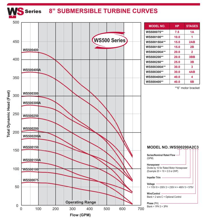
These curves are based on factory tests when pumping clear, fresh, non-aerated water at a temperature not exceeding 85°F. Due to production tolerances, these curves can vary plus or minus five percent.
