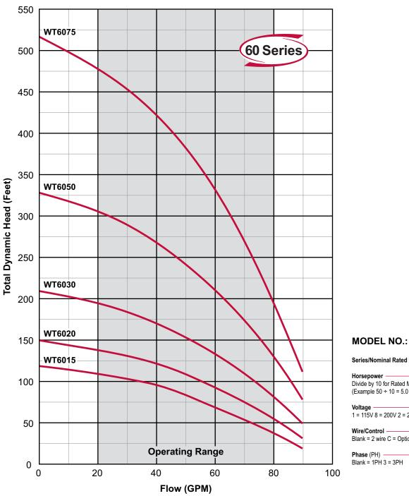
Series/Nominal Rated Flow (GPM) Horsepower Divide by 10 for Rated Motor Horsepower
