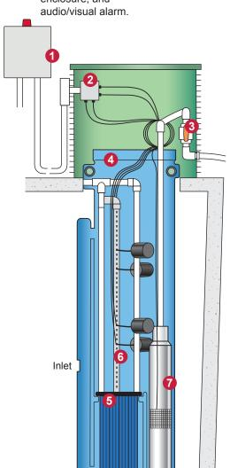
4 Pump Vault An injection molded vault houses the filter assembly. float switches, and effluent pump.
