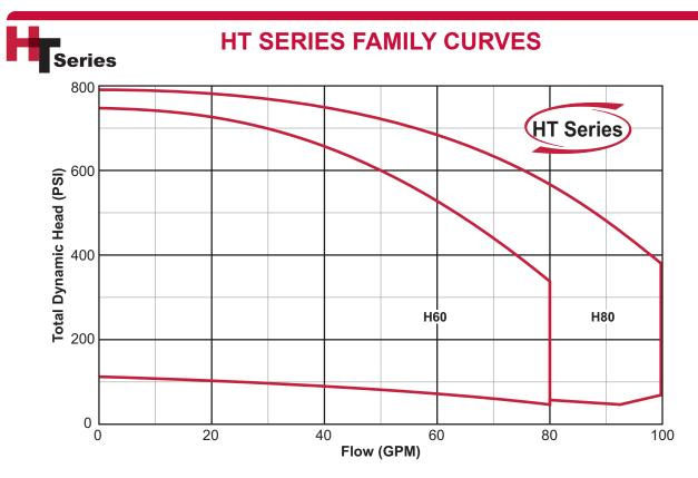
Note: HT Series curves in this catalog are based on 60 Hz 3450 rpm motors. 50 Hz 2875 rpm curves are available. These curves are for general guidance only, individual pump curves are available upon request. A certified curve may be requested for an additional cost. Webtrol will build pumps to fit your specific needs, contact factory for pricing.
